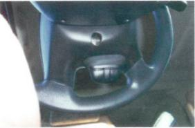
Using the Torx T27 bit, loosen the two screws. Both screws are captive so unscrew them until they feel really loose; you should then be able to lift the airbag module slowly away from the wheel.
