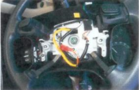
8. The white connector inside the wheel (in the picture above, the one at the top of the wheel) is the connector for the SET/RES switches. At the right-hand side of the wheel you will note the mounting position for the switch bracket. You will need to cut a hole into the plastic trim around the wheel for the switch mounting hardware to pass through, using template supplied
