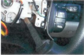
10. As you can see, the bracket that comes with the switch is vital, as is the mounting screw, as the hole for the mounting bracket has been pre-drilled and pre-tapped. You will now need to connect the switch up to the white connector mentioned earlier. Route the wiring so that it goes under the plastic holder and then connects to the plug, which sits back in its rubber holder adjacent to the horn button.
