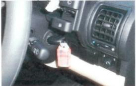
Turn the steering wheel 90 degrees from centre so that one of the airbag securing screws on the back of the wheel is nearest to the floor.
