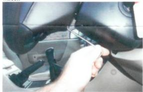
6. The airbag module has a cable connected to it which will allow you to lift the module approx.
