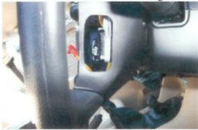
Unfortunately, the hole needs to be quite large to let the lugs on the switch sit up neatly against the plastic. The switch has a nice big rubber gaiter so it's no big deal if the cut is slightly out.
