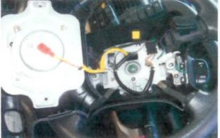
7. To remove the airbag module altogether, simply pull the red connector off the back of it - never pull the wires to unplug any connector, always pull the connector itself. Take extreme care with the module; even though it has discharged by now, it is still an explosive device.
