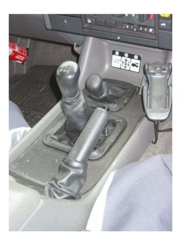
Unbolt gear shift bar from lower lever.
