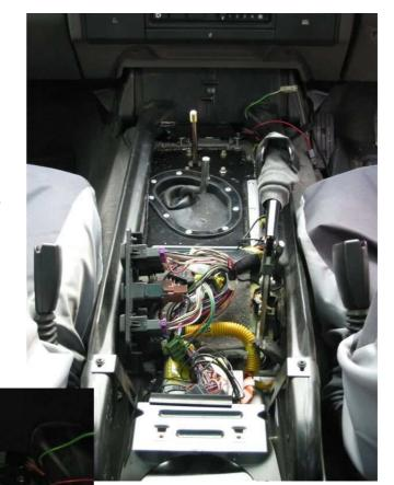
View of the top of the transfer case. The 3 bolts around the CDL spigot have already been removed. Remove the indent spring by unscrewing the cap with an Allen key and hooking it out. Replace the cap. The location can be found next to the arrow in the picture.
